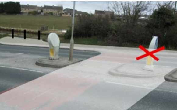
Lengthen central reservation, widen far-side footway and create access to towpath.
