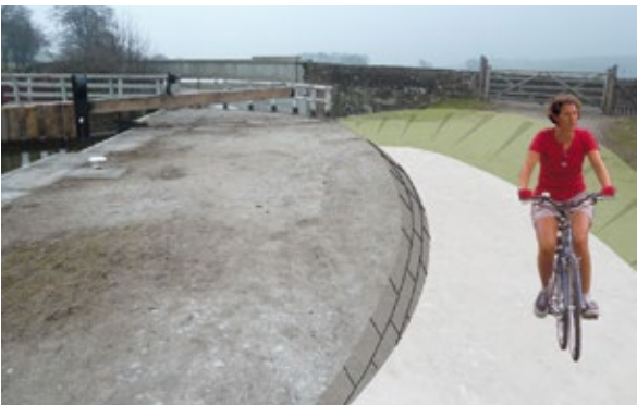
Regrade slope as much as possible to improve gradient, needs further talks with CRT, gate position is new and could be relocated to right of pedestrian gate giving more space for regrading of slope.
