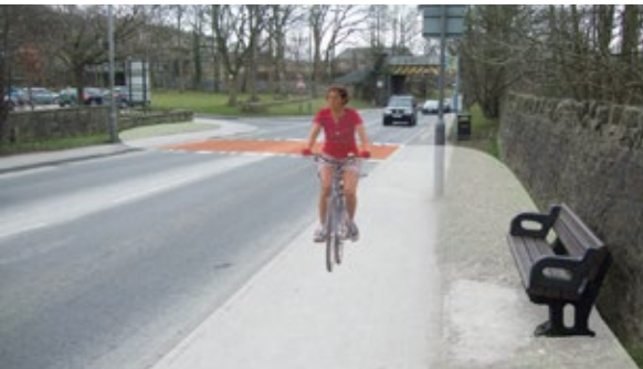
Create dropped kerb crossing point between lamp columns either side, move bench down to bus stop, widen footway to convert to shared use on this side as far as junction behind camera, move sign furniture to back of footway.
