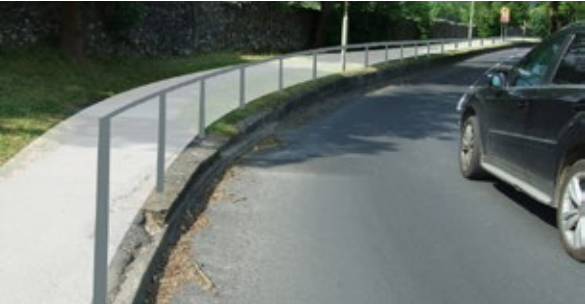
A shared use path could be provided along the footway of Skipton Road to cater for less confident cyclists and families. The mouth of the junction with The Bailey could be slightly reduced to remove the footway pinch point.
