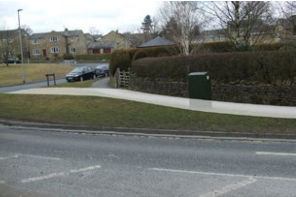
Widen footway to shared use on far side of Gargrave Road to reintroduce to carriageway on Rockwood Drive
