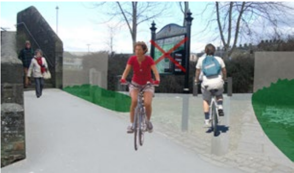
Create new integrated featured access point to towpath, remove vegetation to open up, surface unmade area, relocate bollards and sign.
