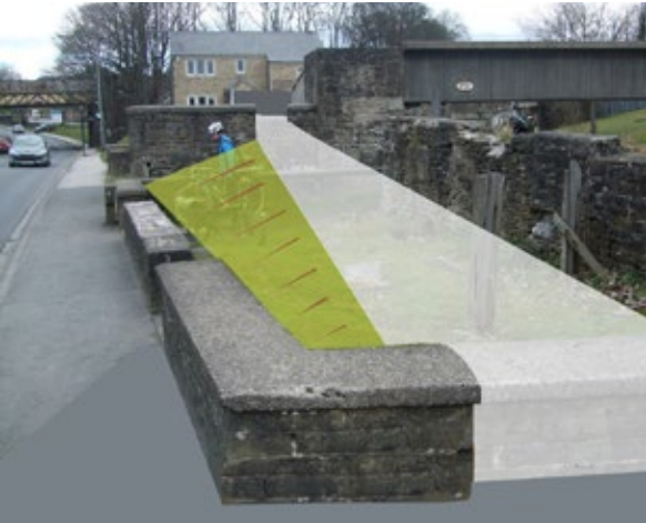
Rearrange ramp approach to bridge, extend and widen middle switchback towards camera through wall next to cyclist and create much better integration between footway, bridge and towpath
