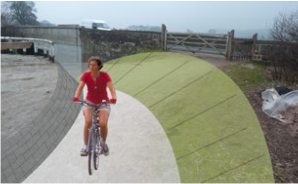
Regrade slope as much as possible to improve gradient, vehicle gate could be relocated to right of pedestrian gate giving more space for regrading of slope.
