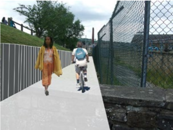
Cut into slope and build new retaining wall to win 2m path width. Improve Rolls Royce fence.
