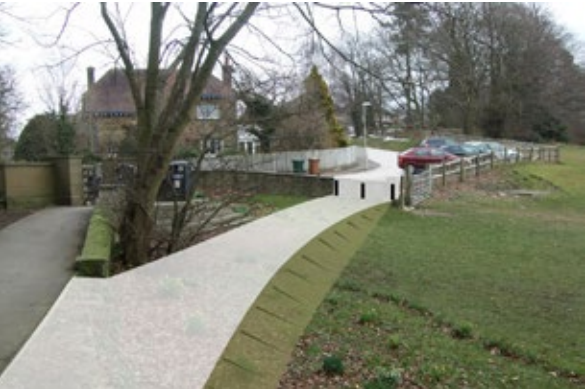
Create new path across to break through wall behind gate, tie-in with bottom of steps, remove low value tree. This serves to deter use of narrow pedestrian access by cyclists
