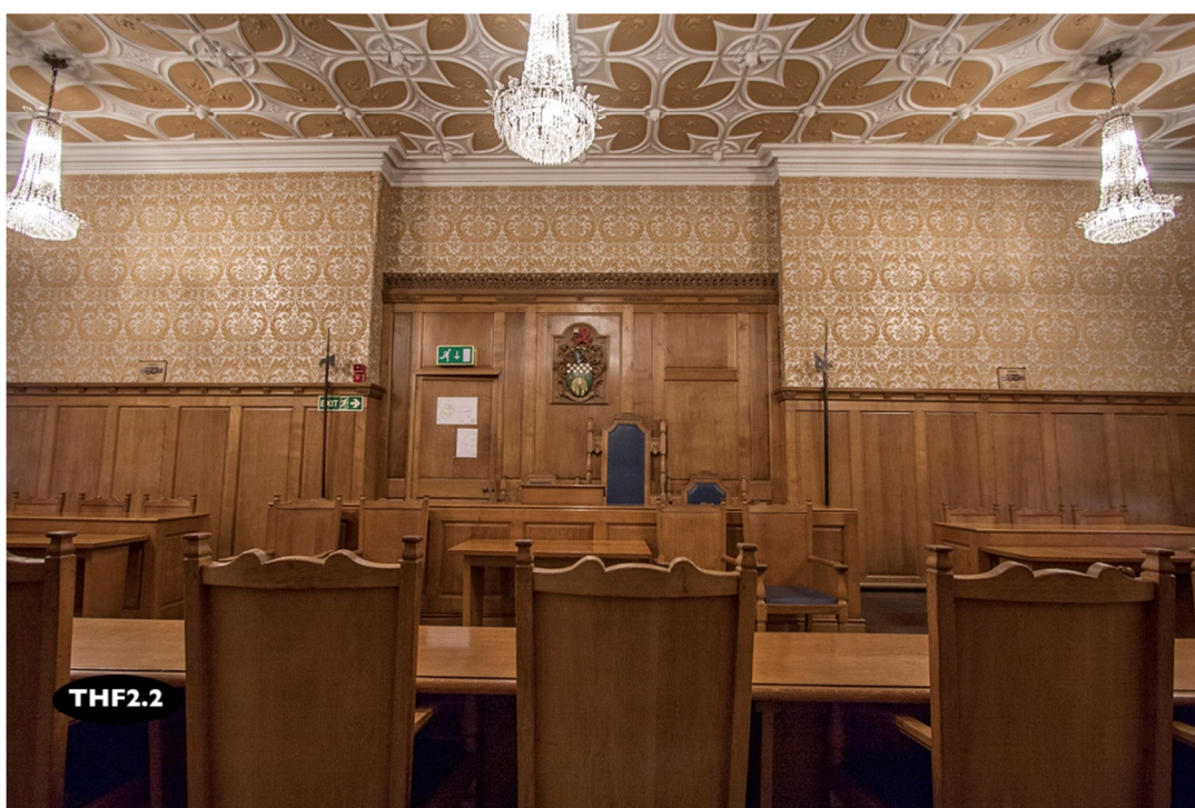
Fig 22 The Town Hall's centenary was marked by extensive alterations. In 1961 the Council Chamber was refurbished, Robert Thompson of Kilburn quoted for delivery and fixing of panelling, platform, lockers, benches, tables, chairs, curtain boxes. The wallpaper and decorative scheme are probably of that date. The ceiling and cornice are probably later 19 th century. Panelling left and right conceals fireplaces and the door leads into the 1838 Big Entry building, taken over entirely for council use by 1963. There is a mouse carved on the back of the right-hand chair. RH
